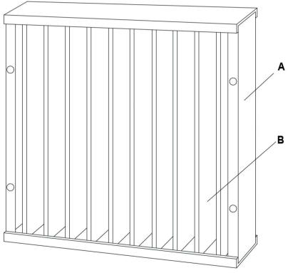
Figure 1. Typical Fire Rated Damper
