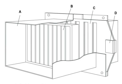
Figure 2. Typical Electro-mechanical Intumescent Damper
